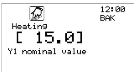
Y1 nominal value defines the first point of the heating or cooling curve as the flow temperature with reference to the setpoint or the reduction value.\*
