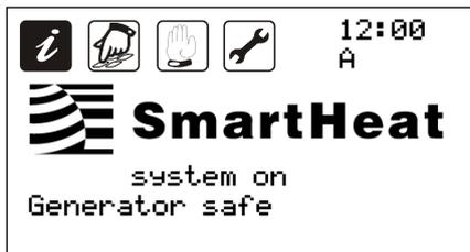
The system has detected a fault in Generator operation. The Generators are disabled by this fault.
