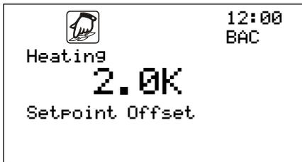
The Offset Setpoint is used to calculate the switch-on and switch-off point relating to a request for heating or cooling
