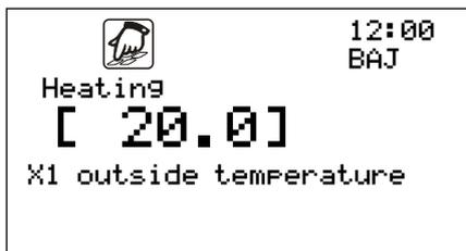
X1 outdoor temperature defines the first point of the heating or cooling curve as the outdoor temperature.\*
