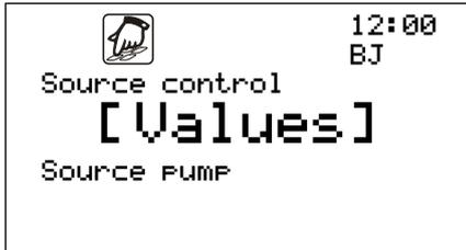
The source control is adjusted in accordance with the machine type and differentiates among different functions and working modes. In this case, Type 2 with pump.
