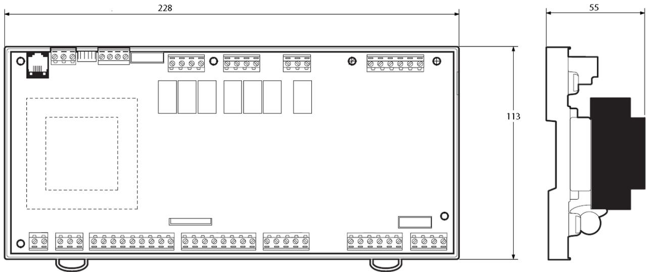
*Figure 4 Control unit dimensions*
