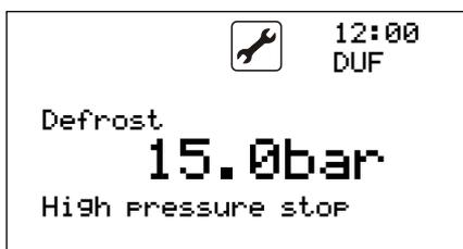
The set high pressure value ends the defrost cycle once the value is reached, though not before the set time has elapsed.
