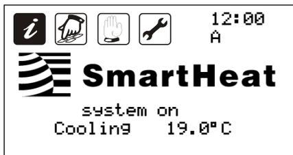
The system is in cooling mode with a setpoint of 19°C.
