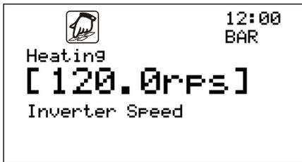
Inverter speed defines the maximum speed at which the function can be carried out. This also serves to limit the power.
