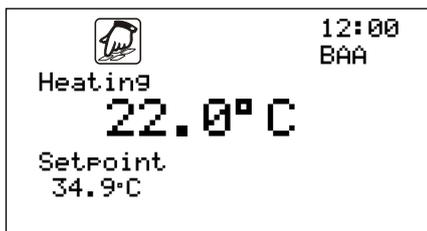
The setpoint relates to a reference value for the flow temperature and indirectly represents the room temperature.
