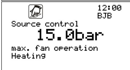
Defining four points establishes a characteristic curve, on the basis of which source control is performed. If the source unit is a pump, it is only possible to define one characteristic curve.
