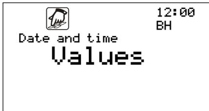
The date and time are entered in the format hh:mm:ss and dd/mm/20yy
