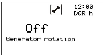
If two, three or four compressors are working as Generators, you can release alternating activation. Then upon each activation, the operating hours are used to determine which Generator to switch on first.
