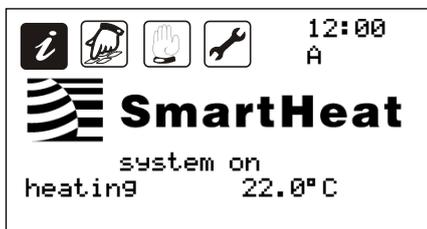
The system is in heating mode with a setpoint of 22°C.
