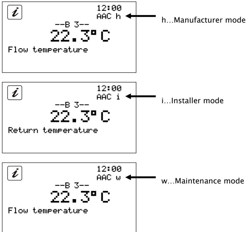
All three modes are activated by entering a password and may only be used by trained specialists, as the wrong settings could cause injury, and damage to the system. No separate character is displayed for the release code.
