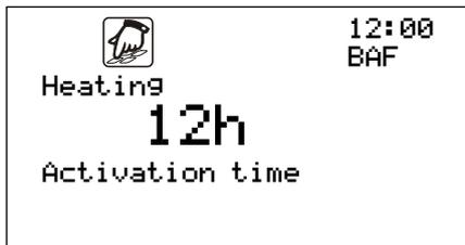
The activation period specifies how long the outdoor temperature must be maintained to enable the heating or cooling function.
