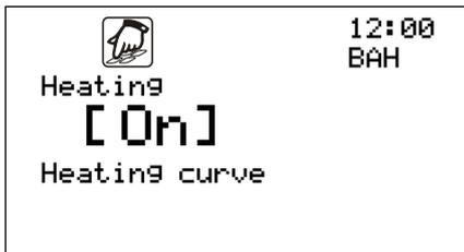
The heating or cooling curve depicts the adaptation of the flow temperature to the current control temperature variable (outdoor temperature or reference room temperature). If the curve is deactivated, a fixed value is used.
