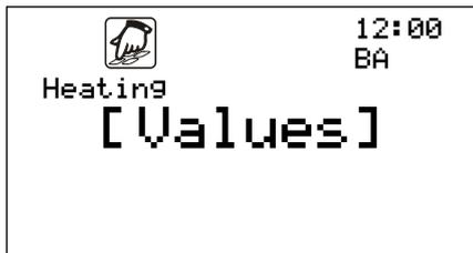
The Heating submenu allows you to programme the functions for heating mode. Certain settings can only be modified if you have the appropriate rights. A password must be entered first. The scope of available settings is the same as for cooling.
