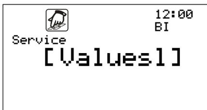
In the Service submenu you can store the telephone number for your service representative, which is shown on the main screen when a disabling message is displayed. This function is not yet available.
