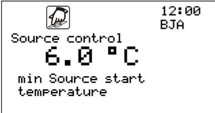
Alternatively, you can regulate the source pump by the source return temperature. This function must be switched on in the "BJN" mask. Then you can parameterize the PID parameters in the following masks and thus influence the control behavior of the pump. The controlled variable is the adjustable minimum source start temperature in the mask "BJA".
