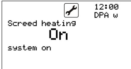
To activate the heating programme, the function is activated (after entering the password).
