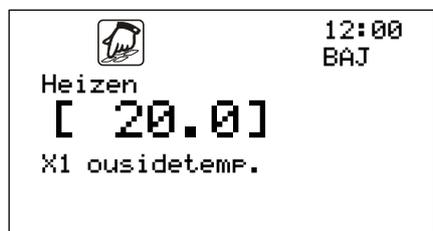
X1 outside temperature define the first point of the heating curve.
