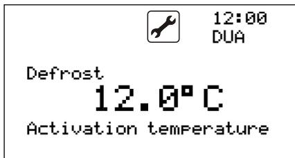
The activation temperature is the outdoor temperature from which the defrost function can be used. The deactivation temperature is the outdoor temperature from which the defrost function can no longer be used. These temperatures define a range within which the defrost function is activated.
