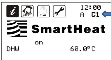
C1 means Unit 1 / Circuit 1
