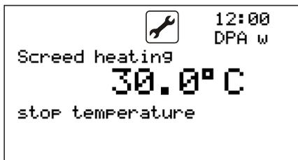
Set the stop temperature, then the system heats back up to the start temperature in this same period.
