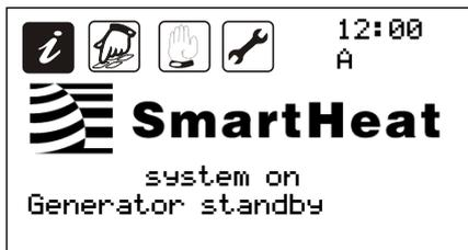
The system does not have a Generator available, possibly blocking time have not yet elapsed or temperature ranges have not yet been reached.
