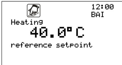
The reference setpoint relates to the flow temperature for a setpoint of 20°C
