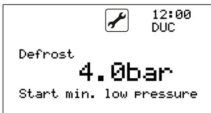
The set low pressure value or temperature difference specifies the operating point from which defrosting should start. The operating point must be present at least for the set control time, in order to fulfil the defrost condition.
