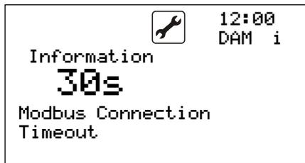
That the monitoring function works, you need to activate it in mask "DAL". After this, the BMS must set all 5-6second a modbus check variable to value true. (see supervisor list). The value will automatically reset to false to check the Modbus connection. Will the Modbus check variable set not set back to "true" then it will occurred a alarm message auf a Alarm delay (Mask "DAM")
