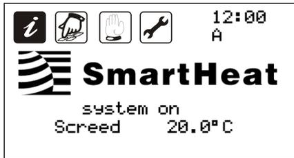
The system is running the screed heating programme, with a current target value of 20°C.
