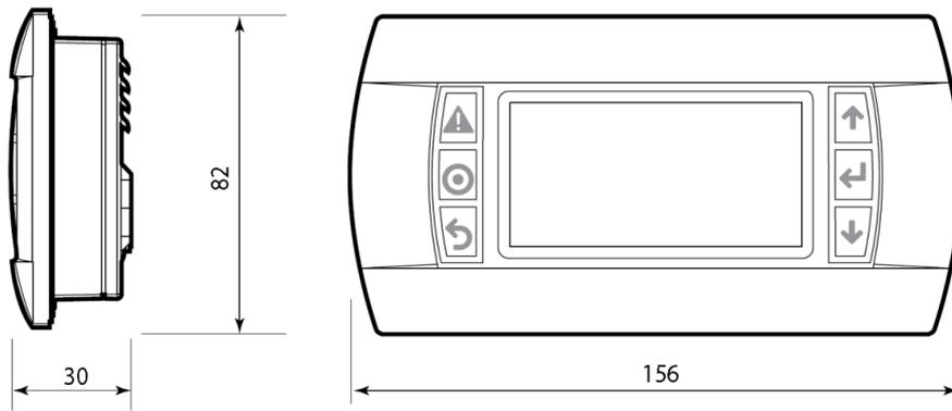
Figure 2 Operating unit dimensions
