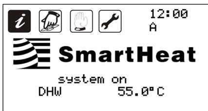
The system is in hot water mode with a setpoint of 55°C.
