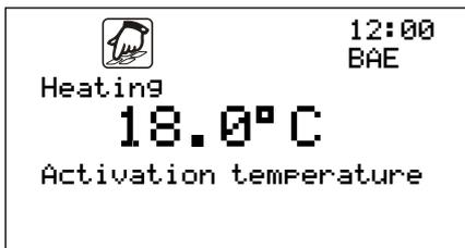
The activation temperature specifies from what outdoor temperature the heating or cooling function is available, according to the activation period.
