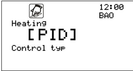
The control type defines the type of speed control for the compressor. The choice of control has a direct influence upon achieving the setpoint. This setting is also important for the cooling function. You can choose from P, PI, and PID.
