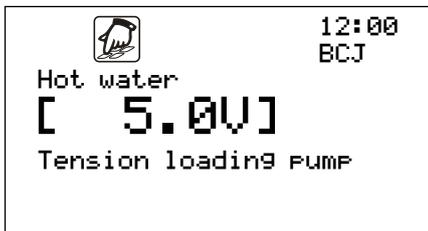
For an output-controlled charging pump, the speed can be adjusted using a continuous signal.
