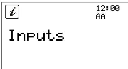
The Inputs submenu shows the values for the analogue and digital inputs. Analogue values include temperatures and pressure values. Digital values include switching statuses of safety devices.
