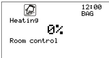
The room control allows the control variable to be switched from outdoor temperature to a reference room temperature.
