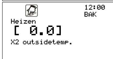
X2 outside temperature define the second point of the heating curve.
