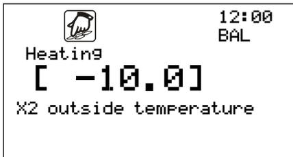
X2 outdoor temperature defines the second point of the heating or cooling curve as the outdoor temperature.\*
