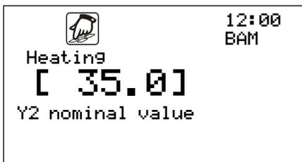
Y2 nominal value defines the first point of the heating or cooling curve as the flow temperature with reference to the setpoint or the reduction value.\*
