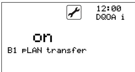
To do this, the pLAN transfer must be switched on in the Options menu under Configuration Inputs.
