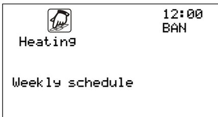
In the weekly schedule two time frames, to which the set target value applies, are defined for each day. Outside of these time frames, the reduction value is applied. The weekly schedule is available for heating, cooling, and hot water.
