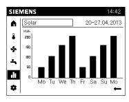
Use the **Energy pages** to compare energy consumption and energy gains (e.g. solar) on a time axis.
