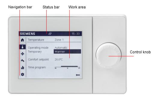
The overview page with navigation bar is displayed when you activate the device. The navigation bar provides for direct access to the main functions.
